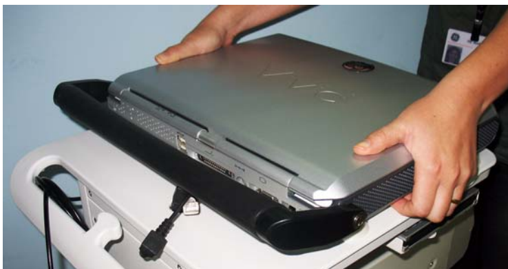
Figure 2-3: Placing on rear sliding guides
