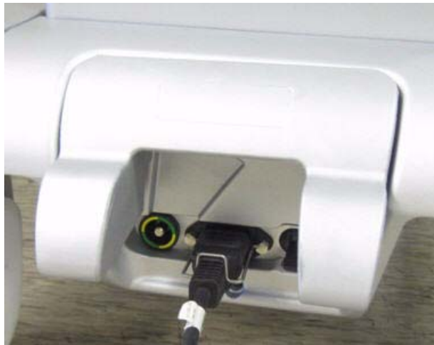
Figure 4-2: Wall-protection for the AC cable
