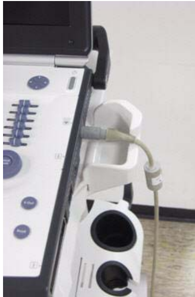
Figure 4-1: Protective support for the ECG connector
